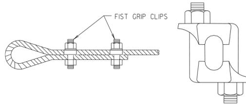
**Description** 5/16" Double-Saddle Fist-Grip Clamp for use with the SafeLink Horizontal Lifeline System. Two pieces per connection required. 5" cable turnback; 30 lbf torque for nuts. Install first clip as close to the loop or thimble as possible. Tighten nuts evenly and alternating until recommended torque is achieved. 2nd clip approximately 1 inch from "dead" end. Always check torque periodically.
